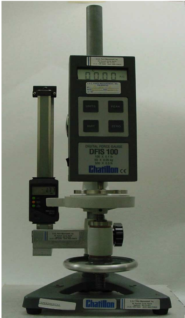
Fig. 1. Chatillon compression decay fixture.
