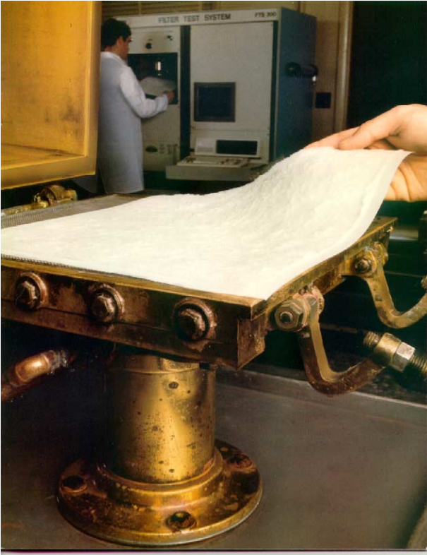
Fig. 3. Handsheet mould, allows prototype laboratory development.
